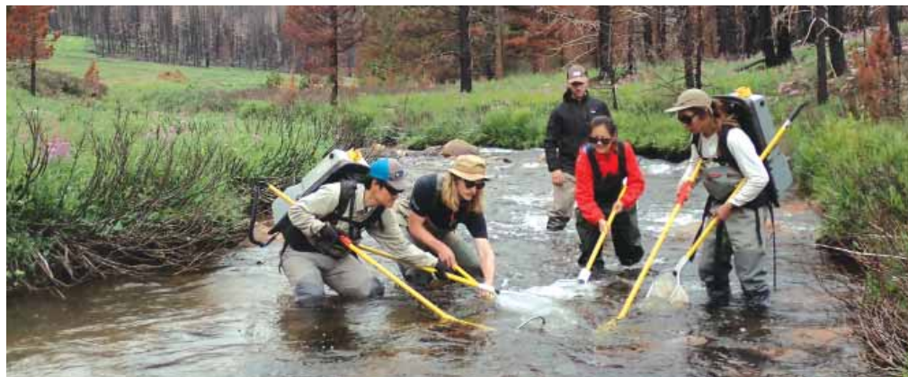
Figure 3. CSU researchers using backpack electroshockers to survey trout. The electroshockers introduce a mild current into the water, which makes the fish easier to catch. The trout are then weighed and measured before release back into the stream where they were caught.
